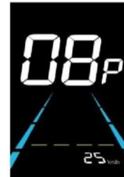
(08P is shown in the picture) Speed limit setting interface
