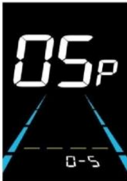
(05P is shown in the picture) Assist gear range setting interface
