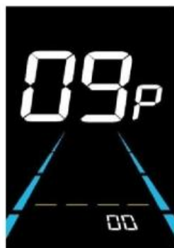
(09P is shown in the picture) Startup mode setting interface
