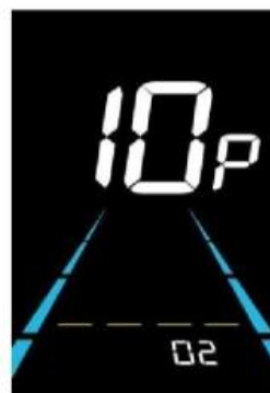
(10P is shown in the picture) Assist mode setting interface
