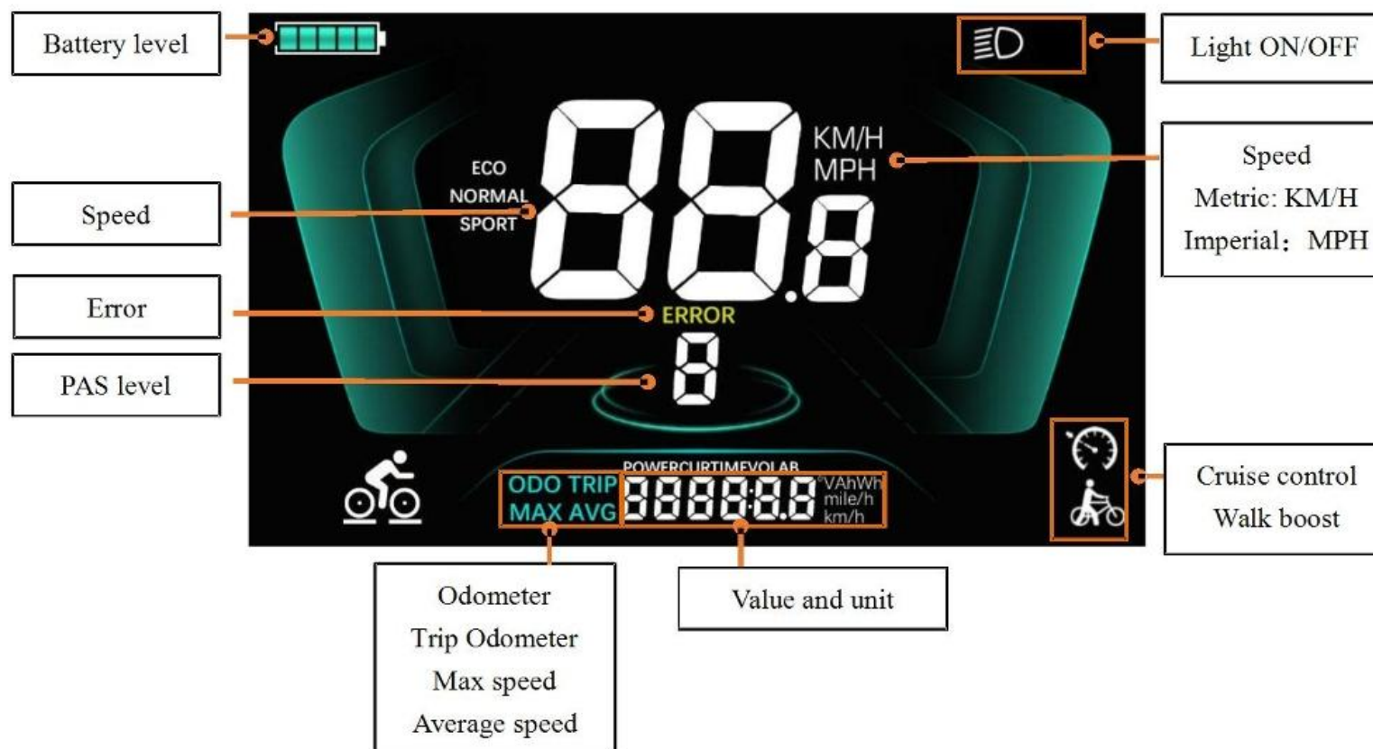
Figure 4-1 YL81F-H functional area distribution interface
